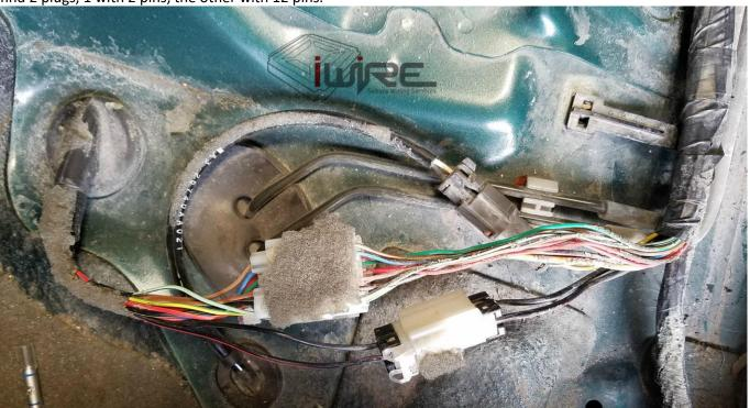
2. Ignore the 12 pin connector, we are going to focus on the 2 pin connector. There is a Black/Red wire and a solid Black wire. **DO NOT CUT THE BLACK/RED WIRE**.
