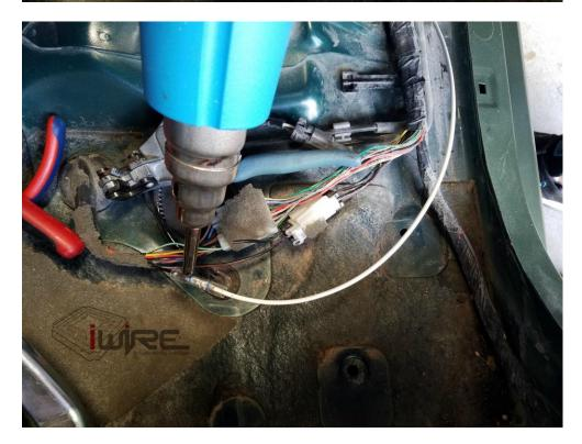
9. To confirm the installation is correct when the key is turned to the on position (assuming the ECU is in and working) the fuel pump will run for a few seconds and then stop.
