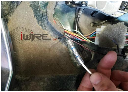
6. Take a set of pliers or crimpers to compress the metal on the Blue line.
