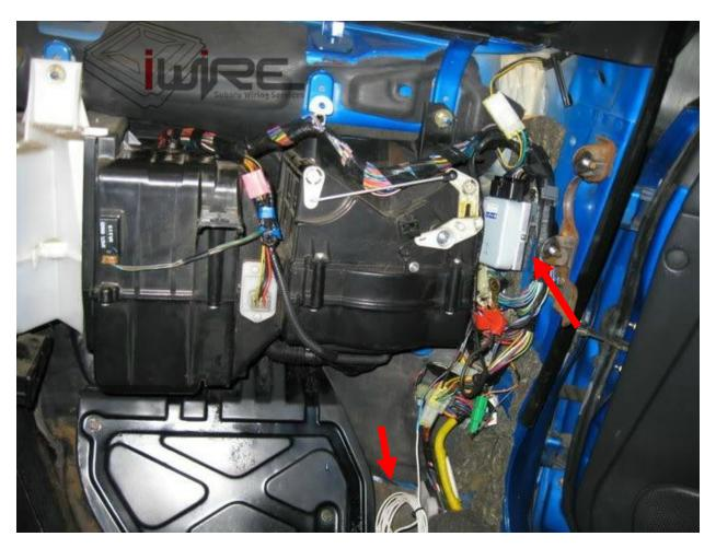
1. First take the White wire to the backseat by running it under the carpet along the door. There you will find 2 plugs, 1 with 2 pins, the other with 12 pins.
