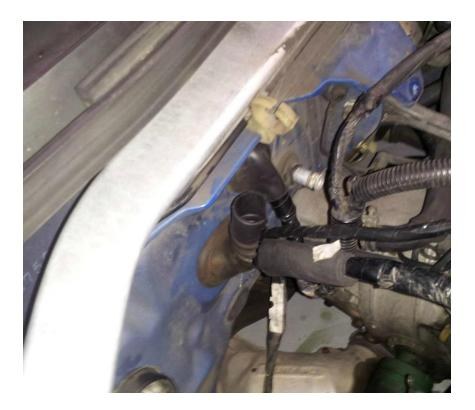
For the section that stays on the on the passenger side you'll notice you may have some extra length of wire, just loop it and tuck the excess in the space between the strut tower and firewall.
