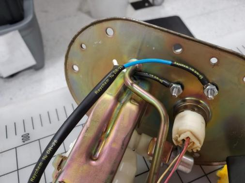
Once the underside of the hanger is complete, flip over the assembly. You'll install the two ring terminals from the main jumper of the iWire FPC Hardwire Kit. **Make sure that the Blue wire is**
