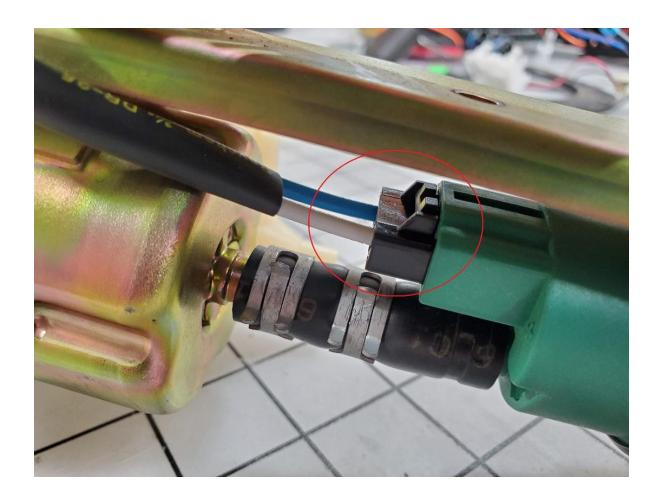
Place the ring terminal from the iWire FPC Hardwire Kit (with the OEM Fuel Pump Connector on the other end) one on each stud on top of the washer. Color order doesn't matter here. You'll just make sure that Blue and Blue touches and White touches White on the same stud. Put the locking nut back onto the stud and tighten, making sure the ring terminal is in place.
