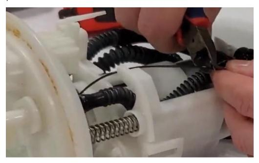
Strip about 6-7mm on each side of the loose wires that will go into the crimp. This wire will be 20 GA.
