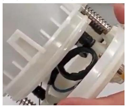
With each kit comes a small metal crimp and piece of plastic shrink tube. You'll use these pieces to connect the black wire from the iWire FPC Hardwire Kit to the Black ground wire on the fuel pump hanger.
