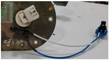
Finally, plug in the black two pin connector to the matching receptacle on the main harness.
