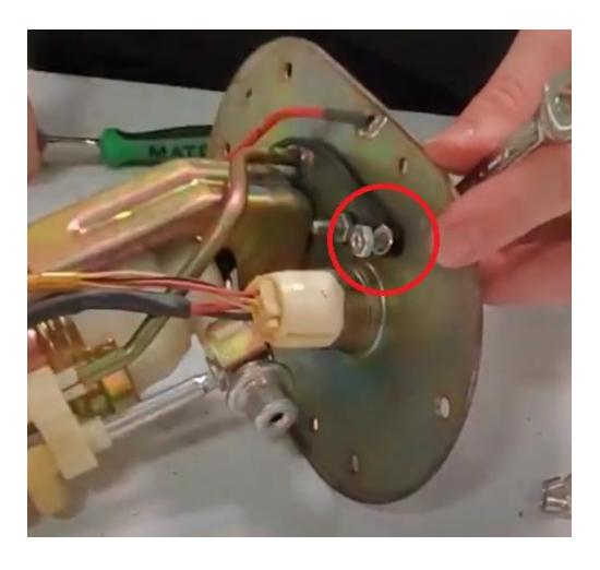
Make sure to route the wire so that it stays within the line of the fuel pump hanger so it goes into the tank once you put the hanger back in and does not get pinched.
