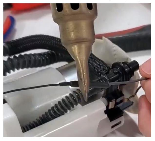
Once the ground wire is complete you'll install the Blue and White wires onto the top side of the hanger following the instructions from Step 3 of the metal hanger install.
