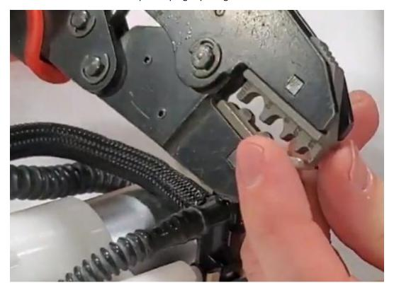
Repeat this step with the second wire and put it into the empty slot of the metal crimp. Crimp tightly. We suggest doing a light pull test to make sure the connection it secure.
