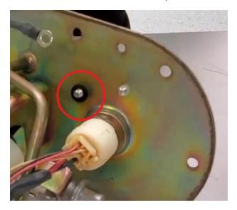
Next, you'll put the locking nut on the underside of the hanger (side of hanger that goes into the gas tank) and tighten it into place. This is done to make sure the insulator is compressed properly. Tighten it
