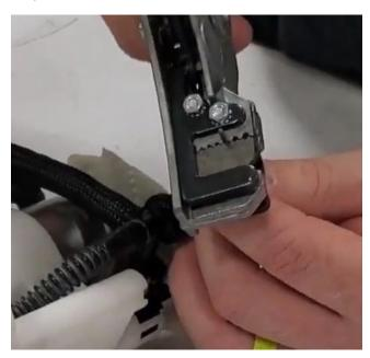
Insert shrink tube onto one of the wires. **(Do this before crimping!)** Then slide one of the stripped wires into one end of the metal crimp. Crimp tightly using a ratchet tool.
