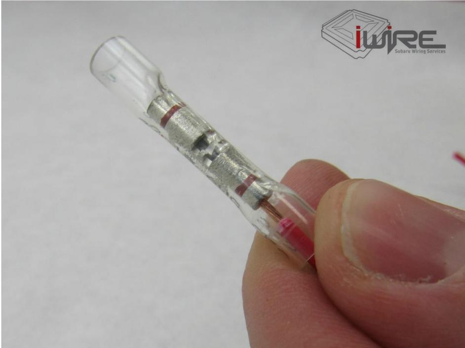
4. For this type of crimp either insulated or non-insulated guides can work. The only concern with the non-insulated section is puncturing the glue shrink sleeve but will result in a better and stronger crimp.
