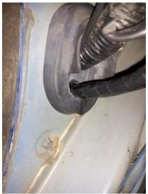
When you pull the engine plugs through the firewall make sure that you pull off the grommet and plastic tubing attached to it. Once everything is lined up then put the grommet back in with the part that sticks out facing up
