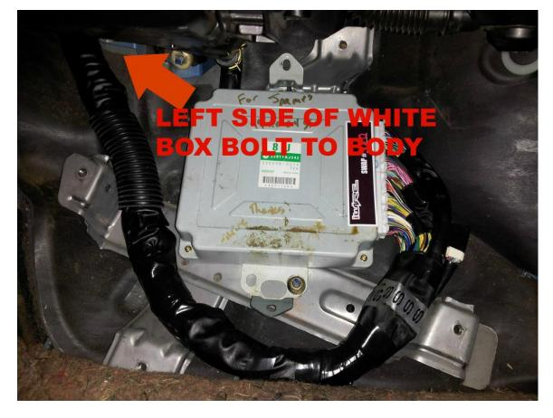
You'll notice the back plate (shaped like an x) has a sharp spot on the left side where the loom goes up. Make sure to slide the plastic cover where the metal is to make sure it doesn't push through at all.
