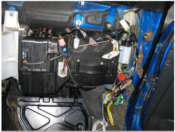
Make sure to secure down the Fuel Pump Controller (looks like big heat sink located by the passenger side door). I usually zip tie it to the harness on that side. Make sure it has a little room to breathe, it gets a little warm, but not hot.
