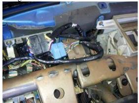
To run the WRX main engine plugs (brown and black (sometimes grey) square plugs) wiring through the fender cut a slit in the grommet on the RS harness that comes through a big oval on the driver's side. When you pull the wires through be careful not to cut them on the chassis, it's pretty sharp. Take the harness and put it above the RS harness over the tabs that stick out to make sure it doesn't come down and rub.
