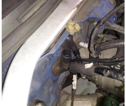
Route the vehicle speed sensor (Black 3 pin) the 2, 2 pin transmission plugs (grey and brown) and the rear o2 sensor (long wires with 4 pins) away from anything hot (transmission is ok). Take the rear 02 plug over the transmission to the driver side and plug in making sure to stay away from heat and secure down. Also make sure the rear o2 sensor (yellow wire from the downpipe) is not going to touch the downpipe. Melted o2s cause serious problems!!
