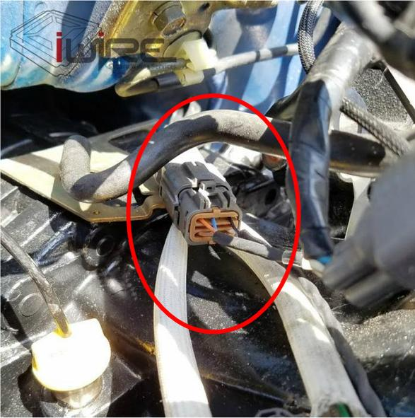
The bulkhead side of the transmission adapter connector plugged in. This will plug into the old transmission wiring from the car's wiring harness. It should be either a single 4 pin plug or two 2 pin plugs. Leave the 3 pin Deutsch connector open for now.
