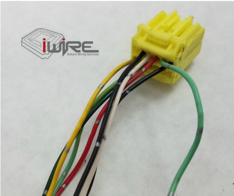
**For V5 to V6 RHD** – Tap into the Light Green wire on pin 20 in the Blue plug for throttle position at the engine computer.
