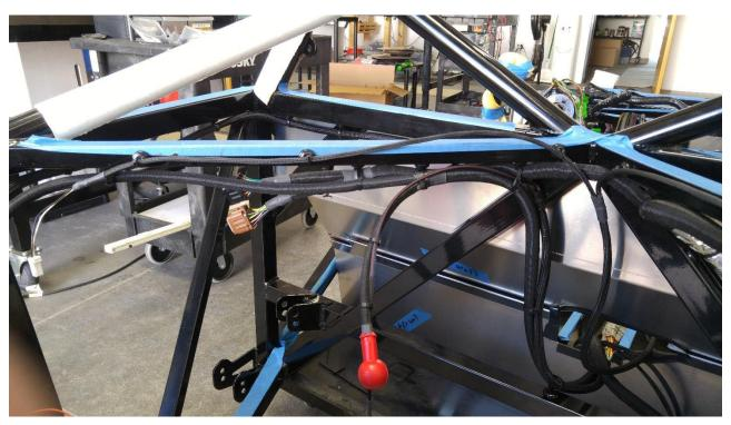
**CB AUX wires** - The smaller alternator wire has a terminal on the end and a tag labeled "CB AUX". This should tie into the circuit breaker on the AUX side with the similarly labeled wire coming off the harness next to the fuse boxes. These two wires get tied together on the AUX terminal of the CB.
