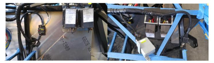
**Dash Section** – The harness should run along the top side of the bracing in order to keep things from falling down to the floor.
