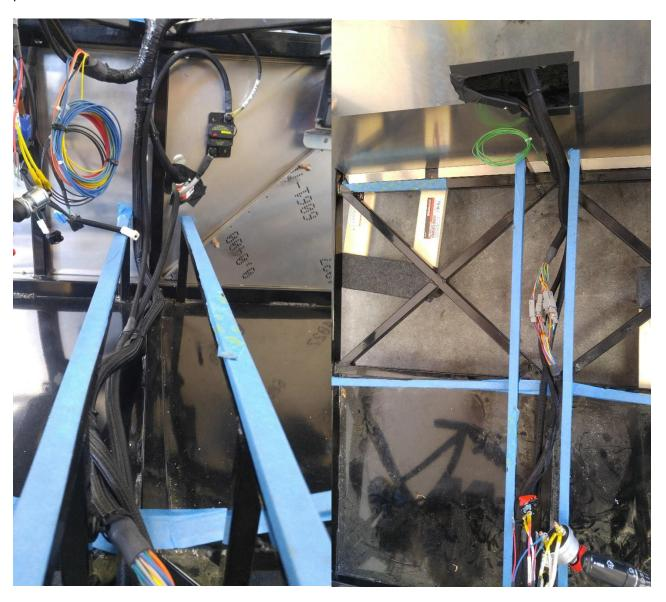
**Front Harness Routing** – The connector plugs from the bulkhead should meet approximately in this spot. Route the harness from the bulkhead out of the firewall hole and straight up to the top where the support bars meet, then run across the driver's side bar to where it will meet the front harness.
