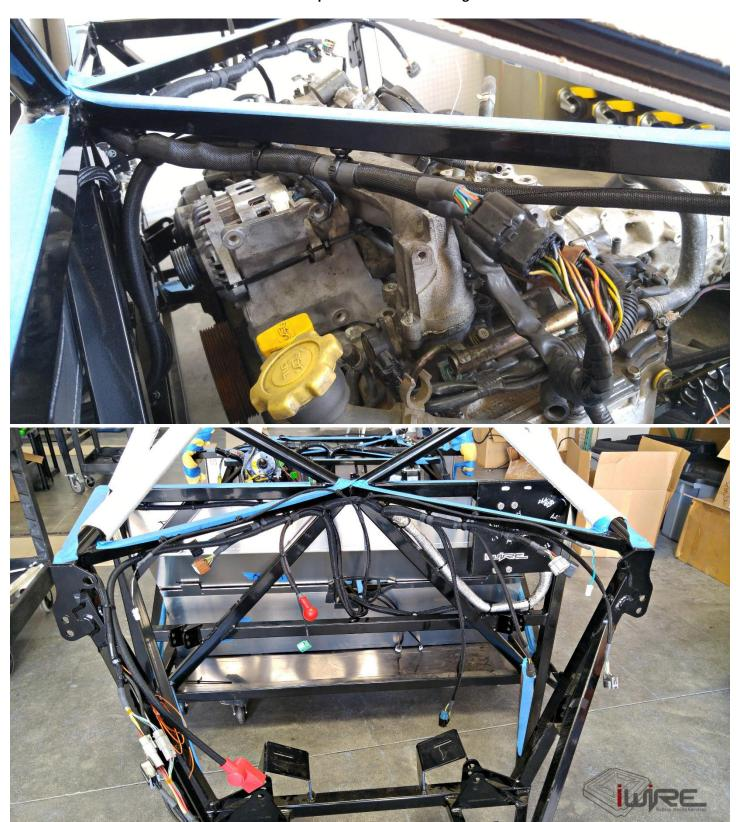
**Rear Harness** – The bulkhead will come up from under the firewall to the top center of the firewall then split toward the driver's side along the underside of the top support beam.
