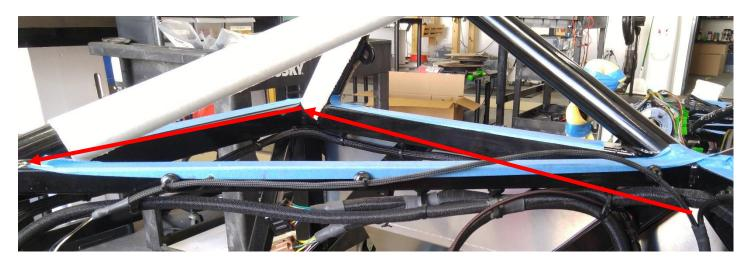
The plugs from the bulkhead and rear harness should meet approximately here. The neutral position/reverse light plug will split where the bottom of the bar and head up to the plug from the transmission.
