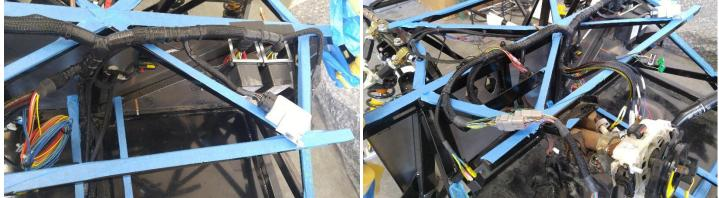
**Center Section** – The main body harness should be mounted on the bottom side of one rail while the alternator/starter sub harness should be mounted on the other to avoid any potential electrical interference from the alternator cable since it generates a fair amount of electrical noise (not the audible kind). It is not required, just recommended if possible.
