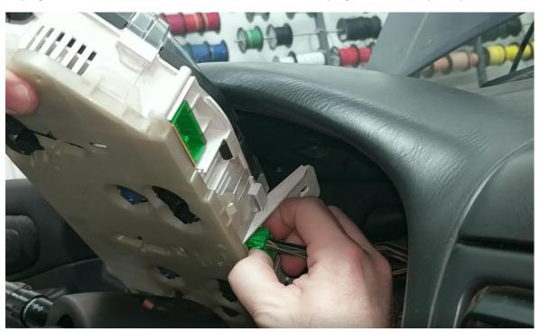
Next you will insert the wires into the cluster plug. First remove the locks on the top and bottom of the cluster plug to install the pins. You can do this with a small pick or screwdriver.
