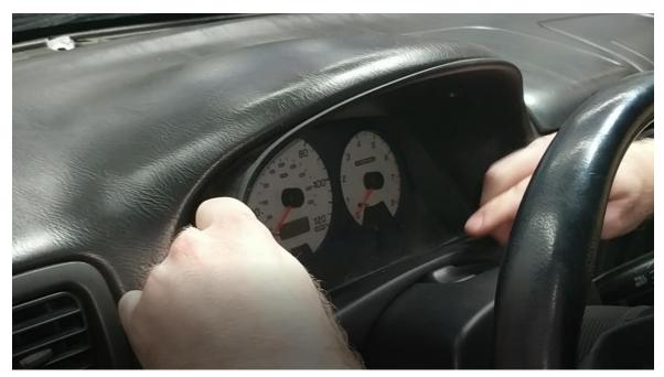
Then unscrew your cluster until you can pull it out slightly and get access to the plugs on the top of the unit. There should be one screw at the top and two screws near each bottom corner.
