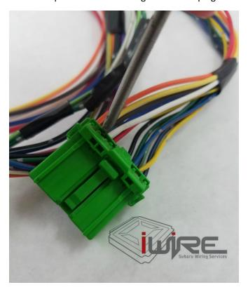
To finish you DCCD Cluster install, plug the cluster plug back into the cluster. Plug the white plug end of the cluster jumper provided in your kit into the matching receptacle on your DCCD. Tuck all of the loose wiring behind the cluster. Reinstall the cluster similar to how you removed it. Plug in all wires, tuck them neatly behind cluster, put cluster back into place and reinsert the three screws, push in bezel surround and reinsert two screws to hold it in place.
