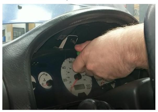
Unplug the needed connector. (see below for which cluster plug is needed for your specific car).
