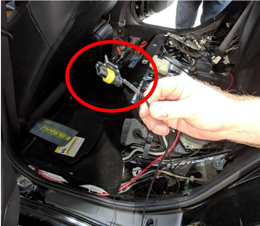
It's best to depin the terminal from the housing. It's the same process as the fuel tank connector.
