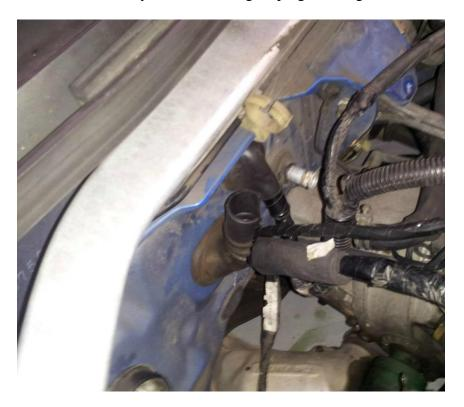
For the section that stays on the on the passenger side you'll notice you may have some extra length of wire, just tuck the excess in the space between the strut tower and firewall.
